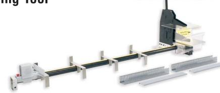
housekeeping associated with power tools. The low cut-force handle speeds product flow while minimizing user fatigue. The tool accommodates left-hand or right-hand setup and features an innovative telescoping measuring bar to suit full-size tables or smaller rolling carts.
