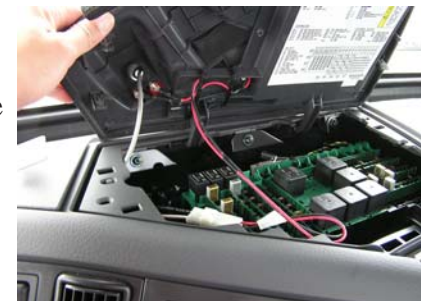
Tilting and Removal of Top
