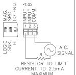
Note: IF EXTERNAL SUPPLY IS USED A.C. SIGNALS OVER 50 VAC PEAK SHOULD BE TO POWER CMOS CIRCUIT VOLTAGE ISOLATED BY A STEP DOWN TRANSFORMER. MUST BE > DC OUT VOLTAGE
