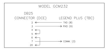
For connection to an RS232 port on a computer, refer to diagrams below.
