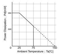
Fig.10 BA6680FS and BD6761FS Power Dissipation Reduction Reduced by 7.6 mW/°C over 25°C, when mounted on a glass epoxy board (70 mm  $\times$  70 mm  $\times$  1.6 mm).
