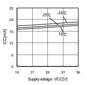
Fig.7 Circuit current (BD6762FV)
