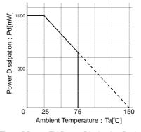
Fig.11 BD6762FV Power Dissipation Reduction Reduced by 8.8 mW/°C over 25°C, when mounted on a glass epoxy board (70 mm  $\times$  70 mm  $\times$  1.6 mm).
