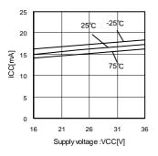
Fig.1 Circuit current (BA6680FS)
