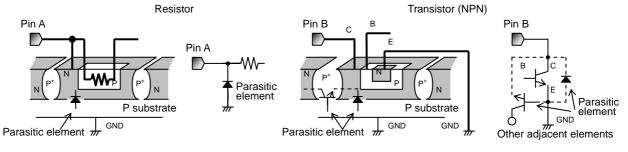
Fig.31 Example of IC structure
