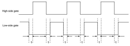
Fig.18 High/Low-side Simultaneous On Prevention Timing Chart
