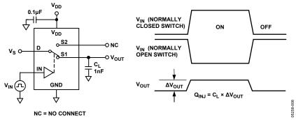
Figure 21. Charge Injection
