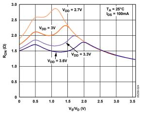
Figure 4. On Resistance vs.  $V_S(V_D)$ ,  $V_{DD} = 2.7 \text{ V to } 3.6 \text{ V}$
