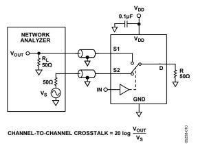
CHANNEL-TO-CHANNEL CROSSTALK = 20 log  $\frac{V_{OUT}}{V_S}$
