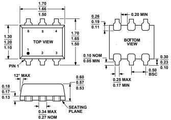
Figure 25. 6-Lead Small Outline Transistor Package [SOT-66] Dimensions shown in millimeters
