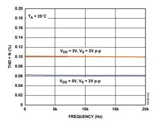
Figure 14. Total Harmonic Distortion + Noise
