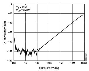
Figure 13. Crosstalk vs. Frequency
