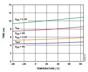
Figure 10.  $t_{ON}/t_{OFF}$  Times vs. Temperature
