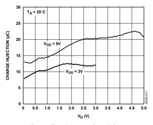
Figure 9. Charge Injection vs. Source Voltage
