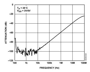
Figure 12. Off Isolation vs. Frequency
