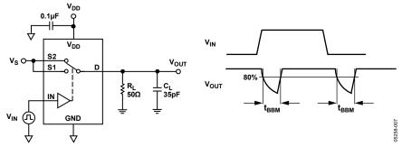
Figure 20. Break-Before-Make Time Delay, tbbm
