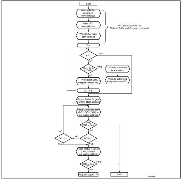
Figure 29. Write to buffer program flowchart and pseudocode
