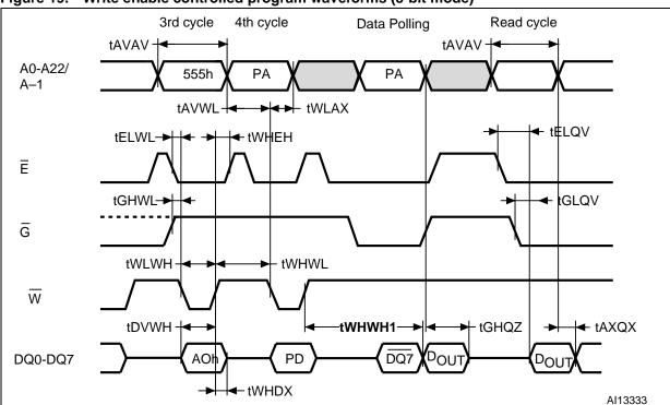
Figure 19. Write enable controlled program waveforms (8-bit mode)
