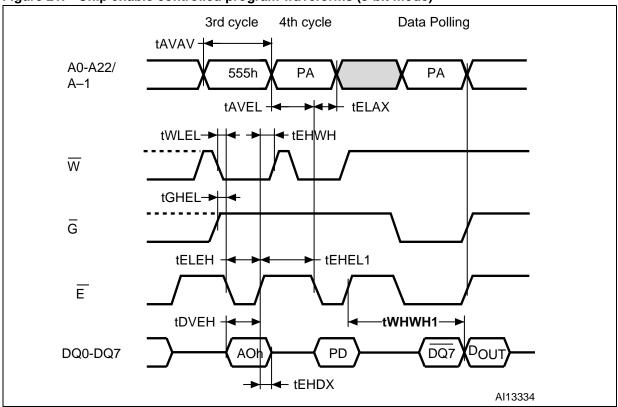
Figure 21. Chip enable controlled program waveforms (8-bit mode)
