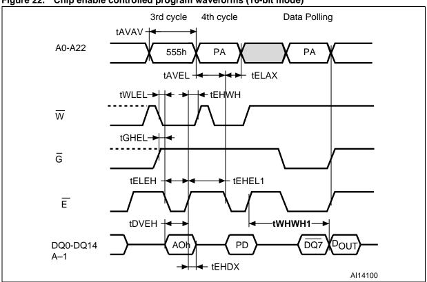
Figure 22. Chip enable controlled program waveforms (16-bit mode)
