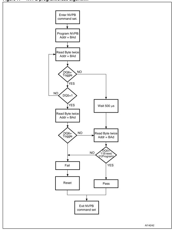
Figure 7. NVPB program/erase algorithm
