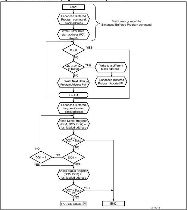
Figure 30. Enhanced buffered program flowchart and pseudocode
