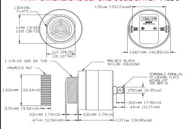
NOTE A: TERMINALS-032 BRASS TIN PLATED, TAPPED FOR #6-32 SCREW. TWO #6-32 NICKEL PLATED BRASS SCREWS INCLUBED. WILL ACCEPT 1/4" OUICK CONNECT. NOTE B: MOUNTING- REMOVE BLACK PLASTIC NUT AND INSERT THREADED FRONT THROUGH 1.25' HOLE PUNCHED IN PANEL, IF DRIENTATION IS NEEDED, NOTE LOCKING FLATS ON DRAWING SCREW NUT BACK ON. DO NOT OVERTIGHTEN.
