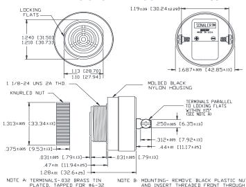
NOTE A: TERMINALS-0.32 BRASS TIN PLATED, TAPPED FOR #6-32 SCREW. TWO #6-32 NICKEL PLATED BRASS SCREWS INCLUBED. WILL ACCEPT 1/4" OUICK CONNECT. NOTE B: MOUNTING- REMOVE BLACK PLASTIC NUT AND INSERT THREADED FRONT THROUGH 1.25' HOLE PUNCHED IN PANEL, IF DRIENTATION IS NEEDED, NOTE LOCKING FLATS ON DRAWING, SCREW NUT BACK ON. DO NOT OVERTIGHTEN.
