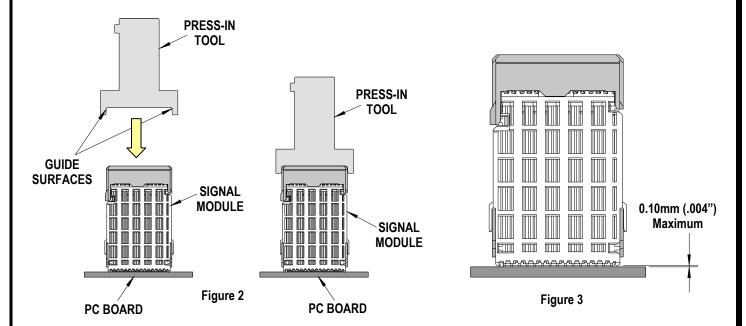
3. Using the application tool and an appropriate press, seat the vertical signal module until there is less than 0.10mm (.004 in) clearance between the bottom of the plastic housing and the surface of the PCB. See Figure 3.
