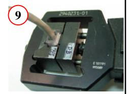
Crimp wires and strain relief
