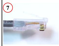
Insert wires and Load Bar into housing
