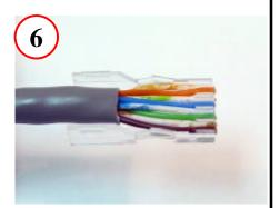
Trim wires flush with end of Load Bar
