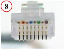
Ensure wires go all the way to front of housing
