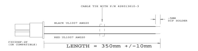
P/N 426013610-3 3MM POWER-IN CABLE 2WAY, 350MM DIGITAL VIEW LTD.
