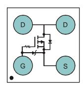
Top View Equivalent Circuit
