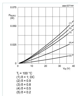
Average reverse power dissipation as a Fig. 7. function of reverse voltage; typical values
