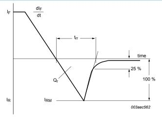
Fig. 12. Reverse recovery definition; ramp recovery
