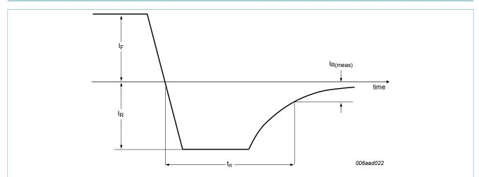
Fig. 11. Reverse recovery definition; step recovery
