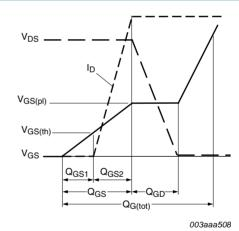
Fig 14. Gate charge waveform definitions
