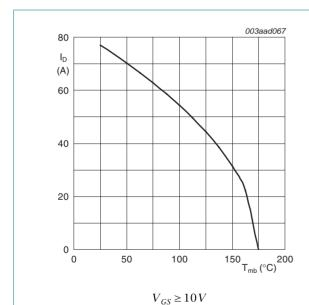
Continuous drain current as a function of mounting base temperature
