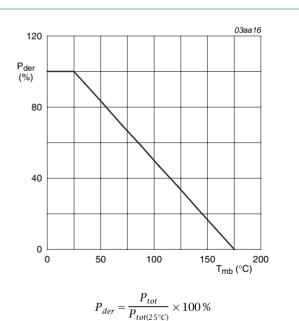
Normalized total power dissipation as a Fig 2. function of mounting base temperature
