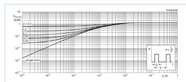
Fig 4. Transient thermal impedance from junction to mounting base as a function of pulse duration; typical
