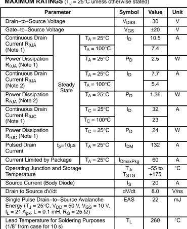
Stresses exceeding those listed in the Maximum Ratings table may damage the device. If any of these limits are exceeded, device functionality should not be
