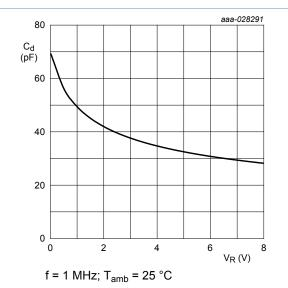
Diode capacitance as a function of reverse Fig. 5. voltage; typical values
