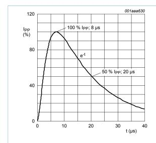
Fig. 2. 8/20 µs pulse waveform according to IEC 61000-4-5
