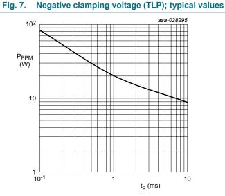
Fig. 9. Peak pulse power as a function of exponential pulse duration; typical values
