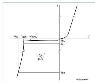
V-I characteristics for unidirectional ESD protection diode
