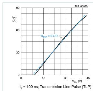
Fig. 6. Positive clamping voltage (TLP); typical values
