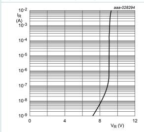
Fig. 8. Reverse current as a function of reverse voltage; typical values
